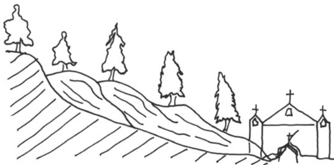
Fig. 3.39 The figure shows successive deep-seated slides with well-defined boundaries but the mechanism is such that trees do not show tilting
