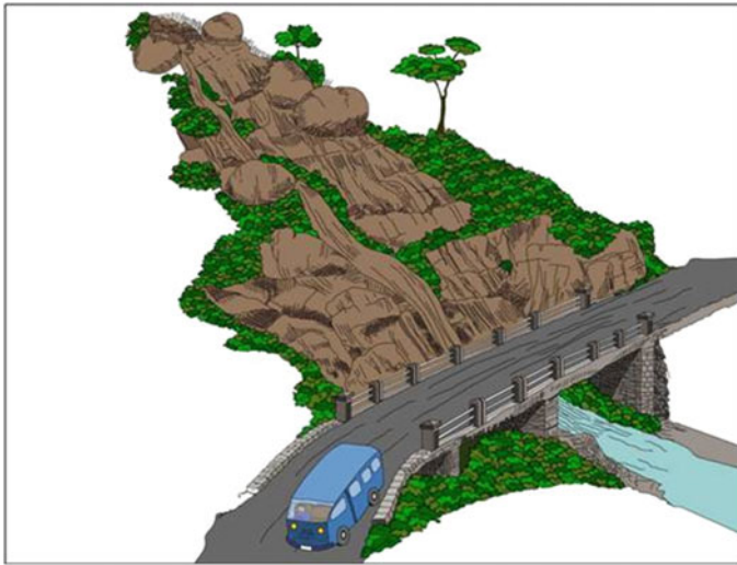
Fig. 3.31 Lyangahawela Bridge in Sri Lanka which was destroyed for the second time by rockfall within a span of about 40 years. Bridges in the rockfall prone areas should be designed to absorb the impact of falling rocks ( Artist Sunil Fernando )
