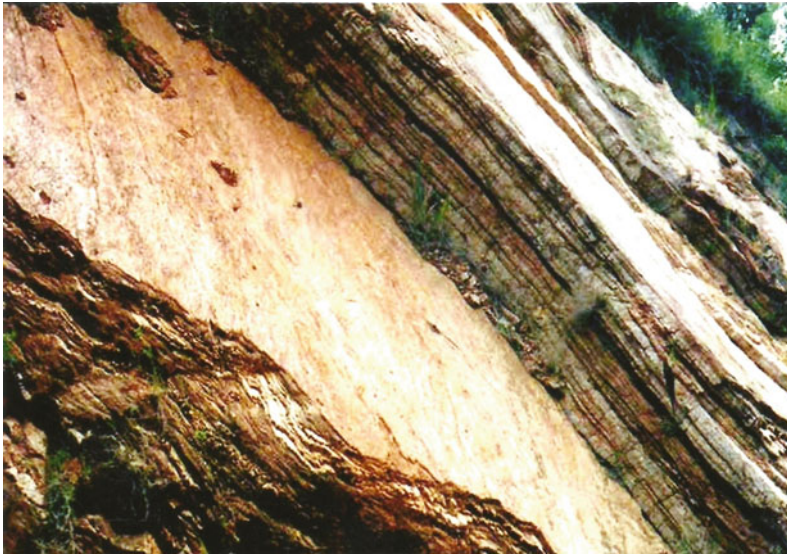
Fig. 3.35 Block and slab slides which occur on discrete boundary shears are known as planar landslides. The point to observe is the unfavorable slope geology which promotes planar slides
